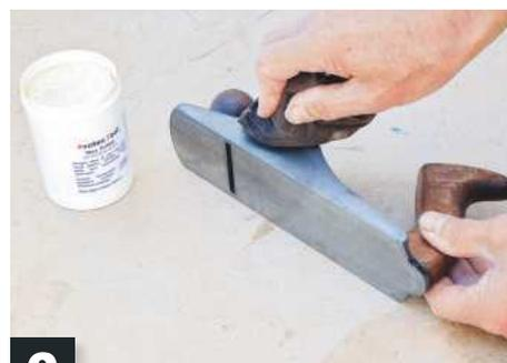
**9** Re-assemble plane and regrind blade. Apply Restore ProtecTool wax or Camellia oil to bare steel surfaces
